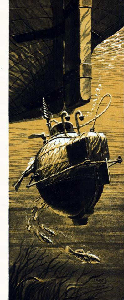
underwater range, would have to approach her target on the surface, probably at night to reduce chances of being sighted. He installed a compass and coated the main points and needle with a phosphorescent, decayed wood called foxfire. The depth-gauge float was similarly marked for visibility in total darkness-probably the first use of luminous instrument dials.
